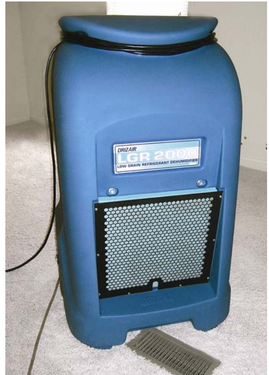
Air conditioner vent feeding air to dehumidifier
